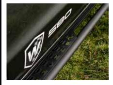
RHINO 4X4 ROCK SLIDERS consist of a solid 3mm material, providing maximum protection while maintaining great clearance. Powder coated matt black and includes high lift jacking points.
