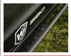
RHINO 4X4 ROCK SLIDERS consist of a solid 3mm material, providing maximum protection while maintaining great clearance. Powder coated matt black and includes high lift jacking points.
